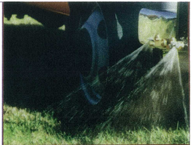
TRUCK-MOUNTED SHORT PATTERN SPRAY NOZZLES
