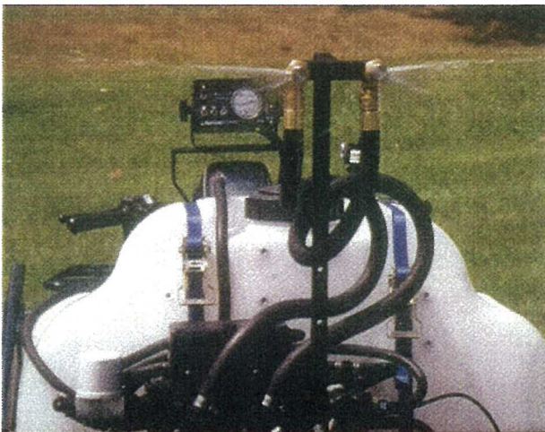
ATV MOUNTED SPRAYER WITH 2 REGULAR PATTERN NOZZLES
